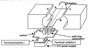
a) Indicate the positive and negative terminals on the DC power supply for this direction of rotation.
