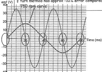
Indicate three times on the graph when the flux enclosed by the coil is a maximum value at 1500 rpm. Circle these times.
