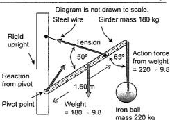
a. Identify all the forces acting on the girder by drawing them on the diagram.
